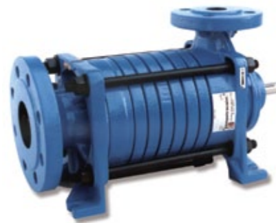
TBA - SELF-PRIMING HIGH-PRESSURE PUMP DESIGN WITH VERY LOW NPSHR CAPABLE OF PUMPING LIQUIDS AT THE BOILING POINT WHILE MINIMIZING THE RISK OF CAVITATION; COMPACT BEARING SHIELD, SHORT SHAFT AND COMPACT DIMENSIONS ELIMINATE VIBRATIONS, WHICH EXTENDS BEARING AND SEAL LIFE.
