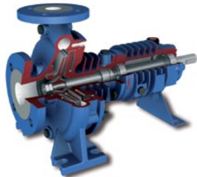
TCD - DESIGN FOR HEAT EXCHANGE OILS UP TO 320 °C WITH SIMPLE MECHANICAL SEALS WITHOUT THE NEED FOR COOLING DERIVED FROM DIN 24258 CHEMICAL PUMP STANDARD; BEARINGS ARE LUBRICATED WITH BEARING OIL AND NOT WITH PUMPED LIQUID AS IN COMPETITOR PRODUCTS.
