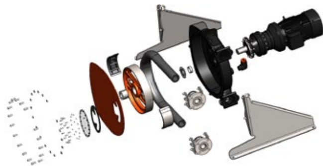
ABAQUE PERISTALTIC PUMP CONSTRUCTION
